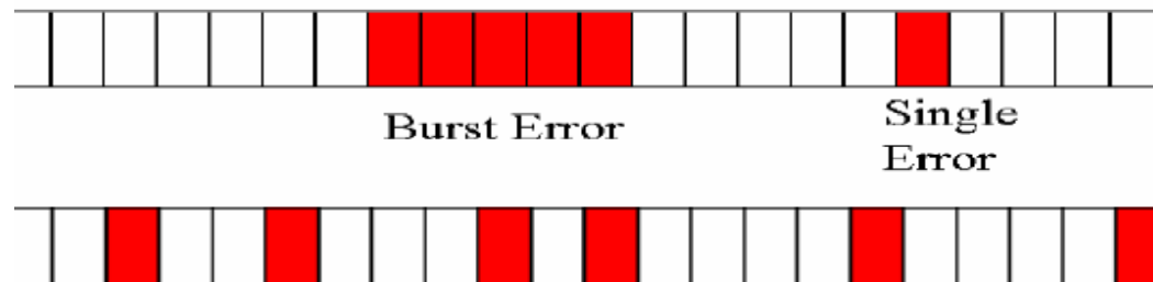
Error Distribution in a Data Signal before and after De-Interleaving
